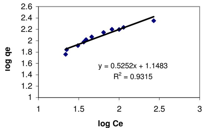
**Figure 8.** The linearized Freundlich adsorption isotherm of direct dye by fungal biomass at pH 5.5 and T = 28 - 30°C.
