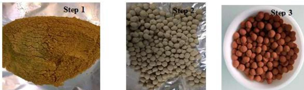
**Figure 1.** Steps in the manufacture of calcined clay beads.
