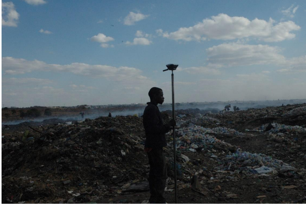
Figure 3. An EMLID Rover is held in place to collect GCP at Chunga Landfill.
