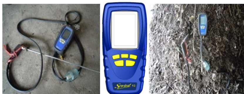
Figure 6. Device for measuring the oxygen level.
