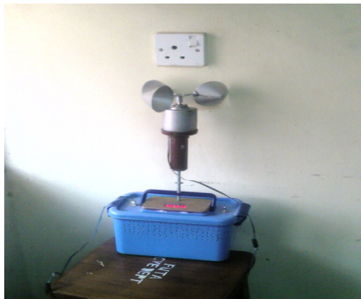
Figure 5. Pictorial view of the developed cup anemometer.
