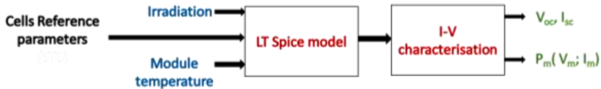
Figure 3. Illustrative diagrams of the inputs and outputs of the LTSpice model.
