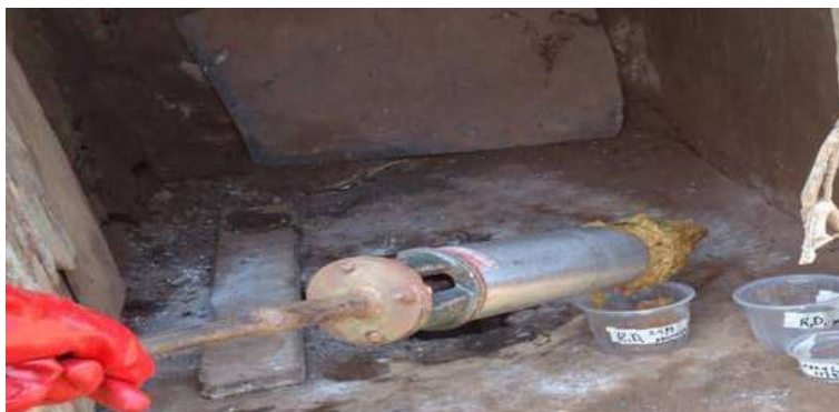
Figure 2. Sludge sampling using a manual sampling tool.
