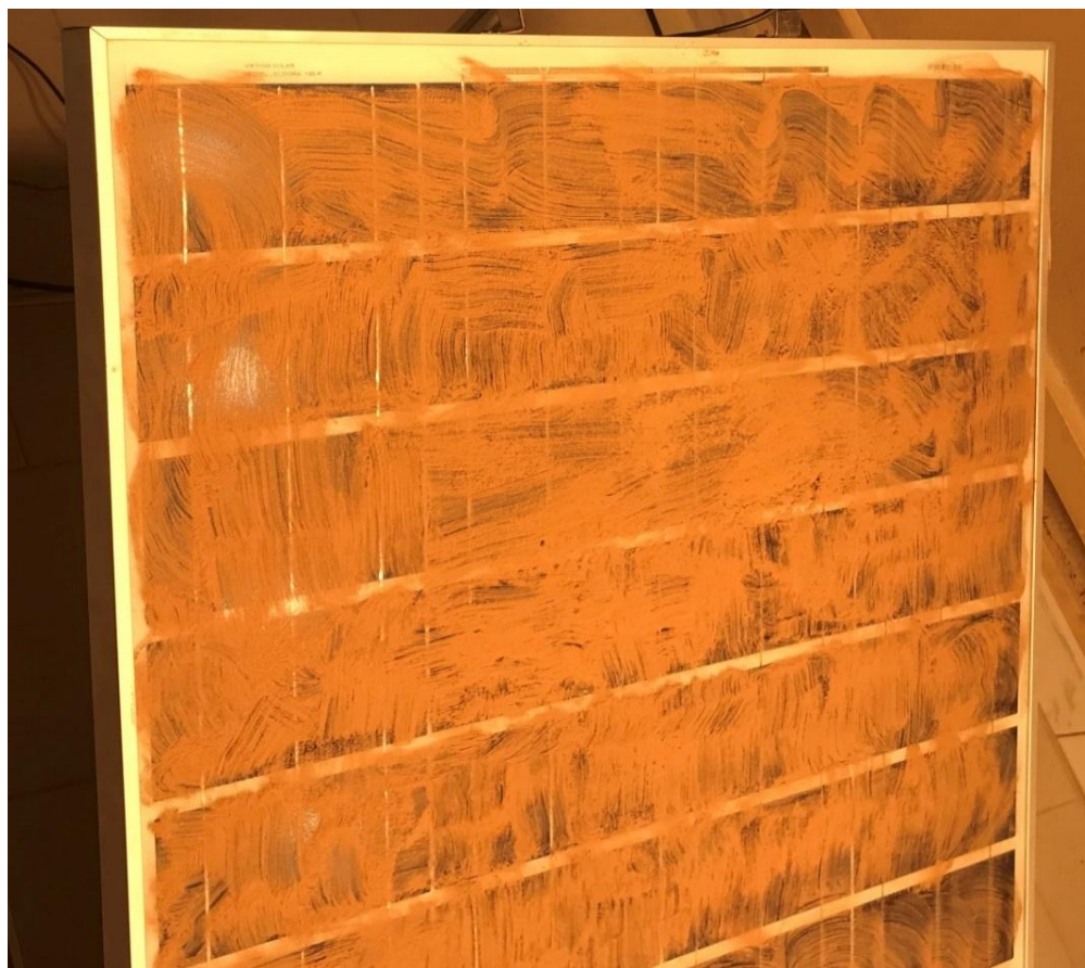
Figure 19. 3rd year of deposit accumulation on the polycrystalline PV panel. Source: Author
