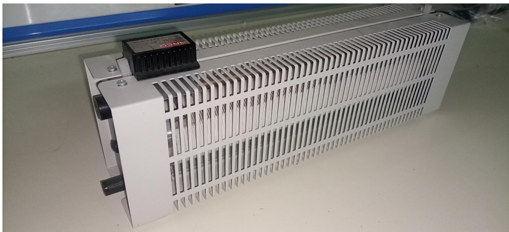
Figure 4. Perspective view of a rheostat. Source: Author
