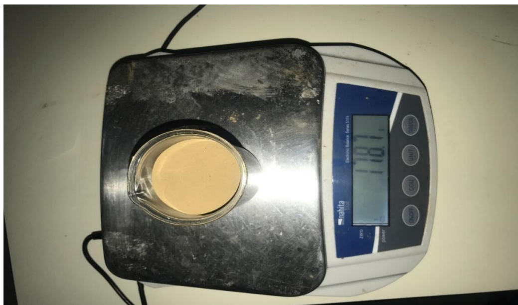
Figure 7. Top view of the precision balance on which the low-profile graduated beaker containing dust is placed. Source: Author
