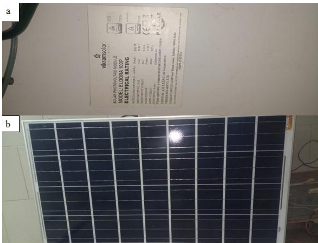
Figure 6. 100 W polycrystalline photovoltaic solar panel: (a) bottom view, (b) top view. Source: Author
