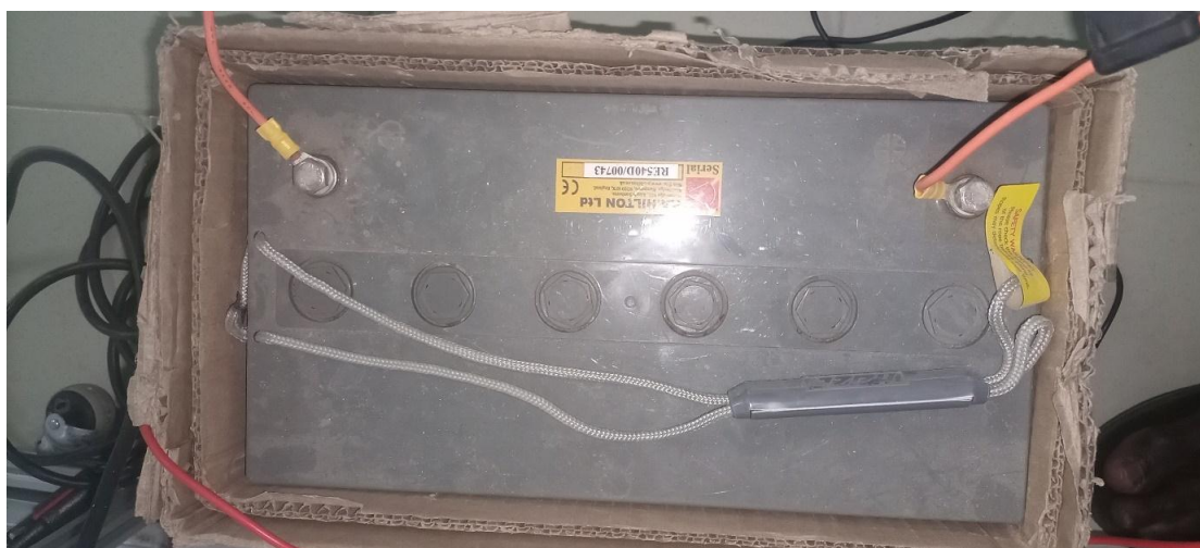
Figure 5. AGM Series 3 battery used in our study. Source: Author
