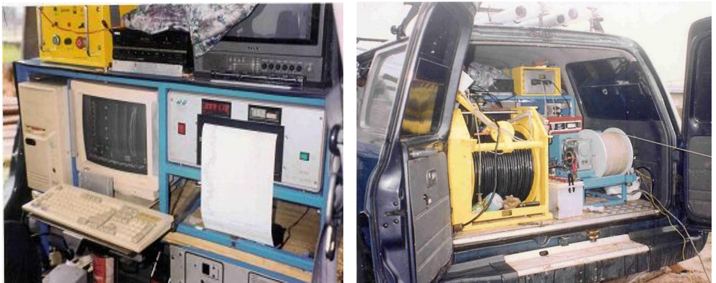
Plate 1. The RG PC Logger II™ Unit mounted on sports utility vehicle used for borehole loggings utilized for the study.
