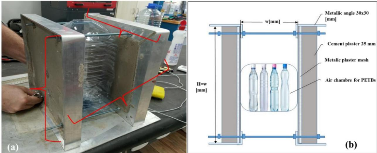
**Figure 2.** (a) Metal frame panel prototype with (H=W=300 mm); (b) PETB metal frame panel prototype with plastering cement; PETBs<sup>ar</sup> panel prototype for thermal tests (Cross-section) adjustable from 114 to 250 mm. Source: Authors.
