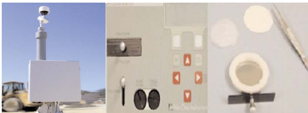
Figure 1. Filter loading area of the E-Sampler (Model 9800 Rev G).
