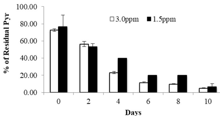
**Figure 5.** Percentage of residual Pyr remaining over time in the culture media during incubation in the dark with 3.0 and 1.5 ppm of Pyr at 30°C, pH 7.0 and at 180 rpm). Each data point represents the mean  $\pm$  standard error of three replicates.
