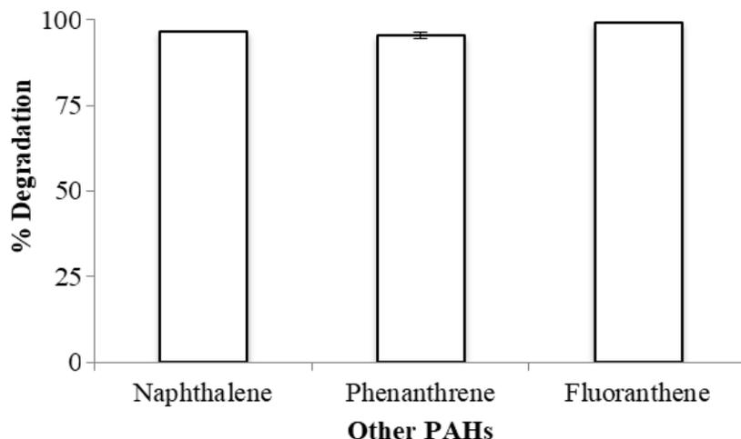
**Figure 7.** Percentage degradation of naphthalene, phenanthrene and fluoranthene at a concentrations of 0.86, 1 and 1.38 ppm, respectively. Each data point represents the mean of two replicates.
