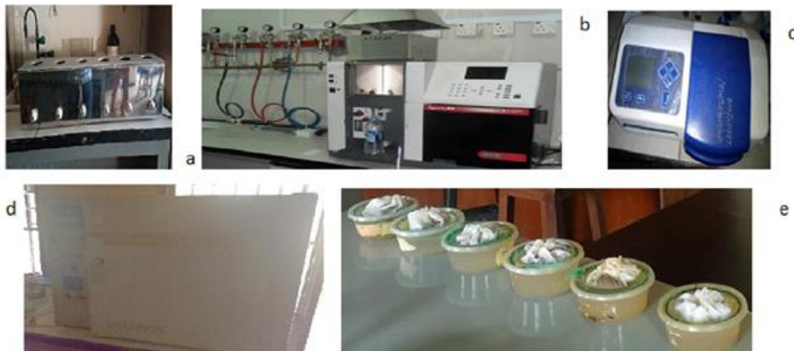
Plate 1. a: Kelgdahl digester (Gallekemp digester); b: SpectrAA55B Atomic Absorption Spectrometer c: Jenway 6305 Spectrophotometer, d: +2 Gallekemp oven, and e: Modified Bearmanns soil extraction set-up for mobile soil nematodes.
