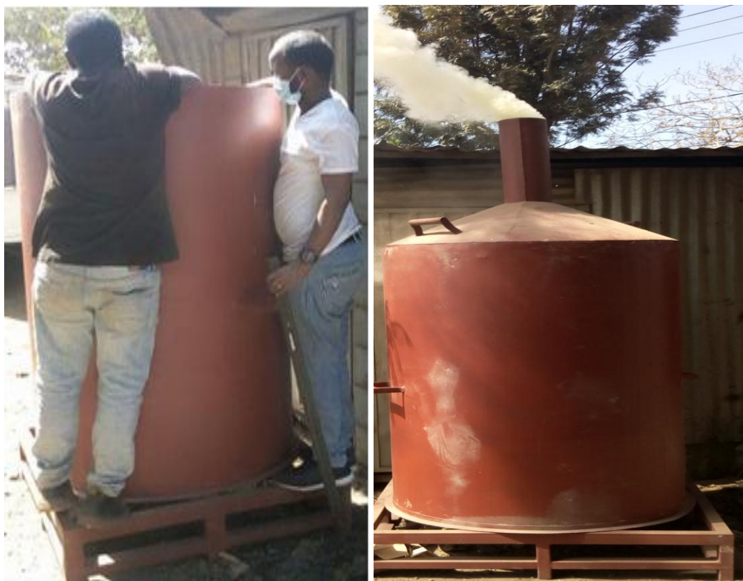
Figure 3. Metal barrel-kiln carbonization machine.
