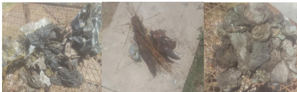
Figure 6. Examples of some constituents from the fractionated solid waste (Left: Plastics; Middle: organic waste; Right: Textiles (note the high content of diapers within the textile component), Kanyama study area.
