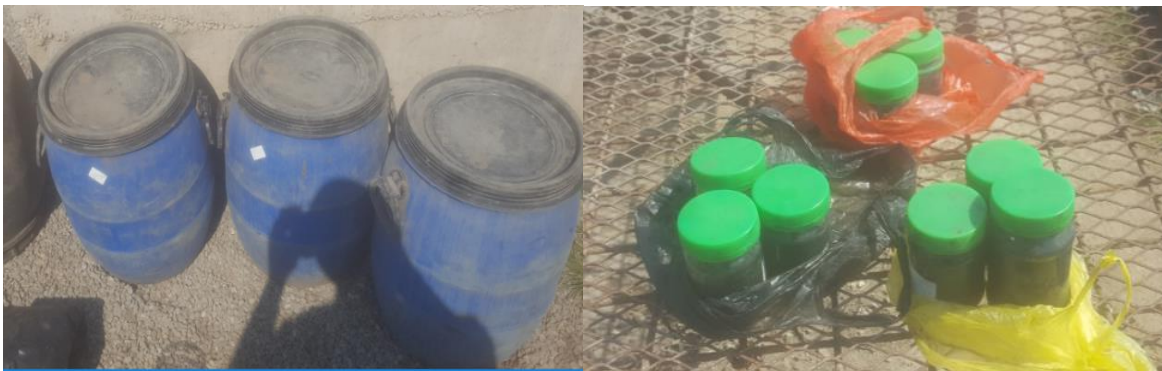
Figure 3. Faecal sludge sampling for analysis (Left: Collection of three 60 liter barrels per Pit latrine; Right: Three samples collected from each barrel for Moisture Content analysis).
