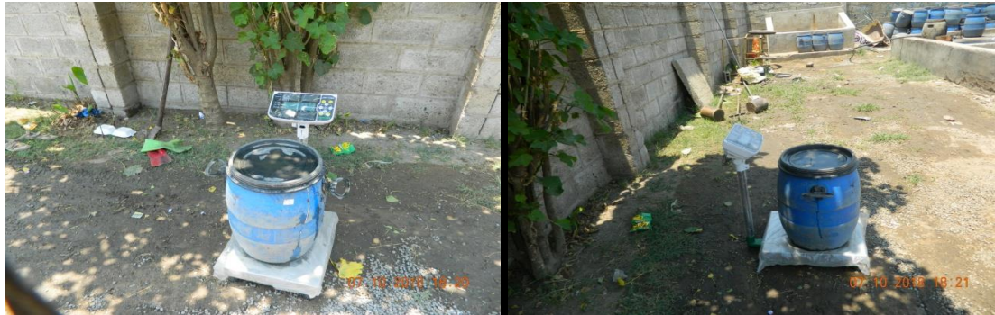
Figure 4. Weighing of the barrel together with the faecal sludge before separation, Kanyama study area.
