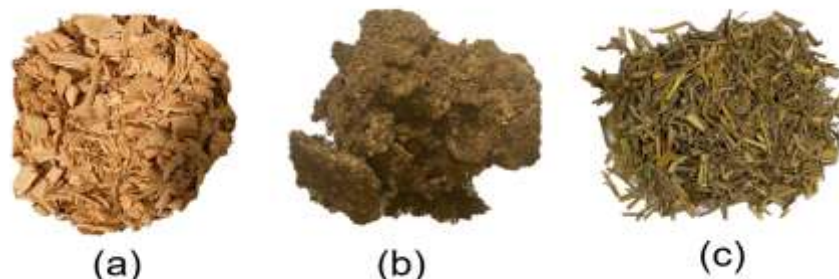
Figure 2. The biomass samples (a) pine wood (b) poultry litter and (c) rice straw. Source: Authors
