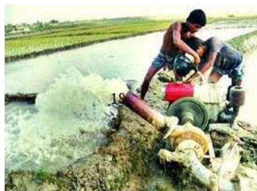
Figure 44. Irrigation by shallow tubewells from a depth of about 30 m (Courtesy of Banglapedia, 2021b)
