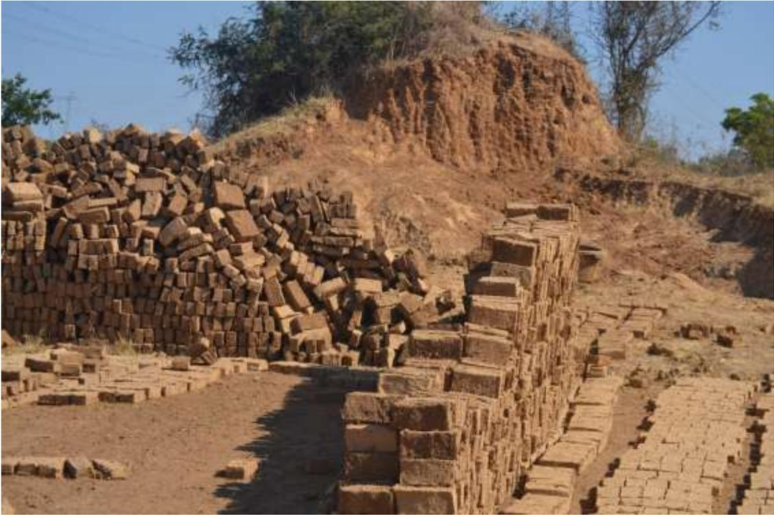
**Figure 5.** Moulded clay bricks before they are baked in kilns.
