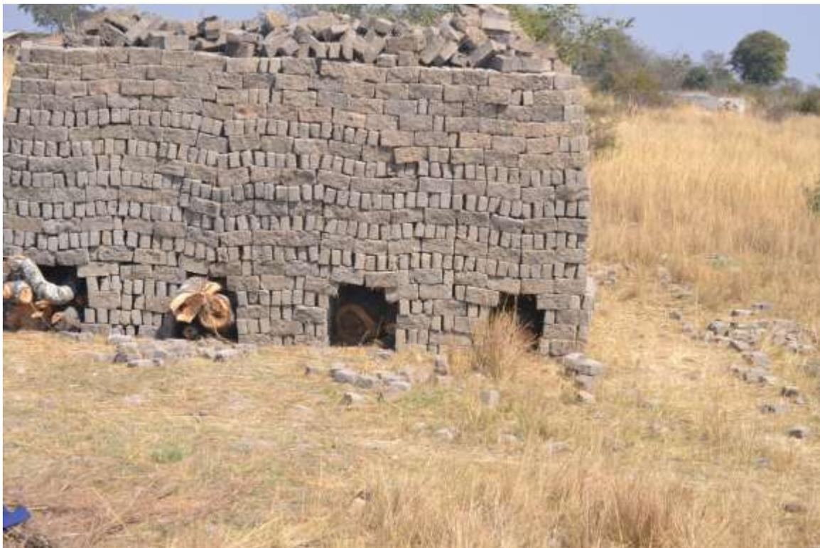
**Figure 6.** Example of a Kiln for baking moulded brick.
