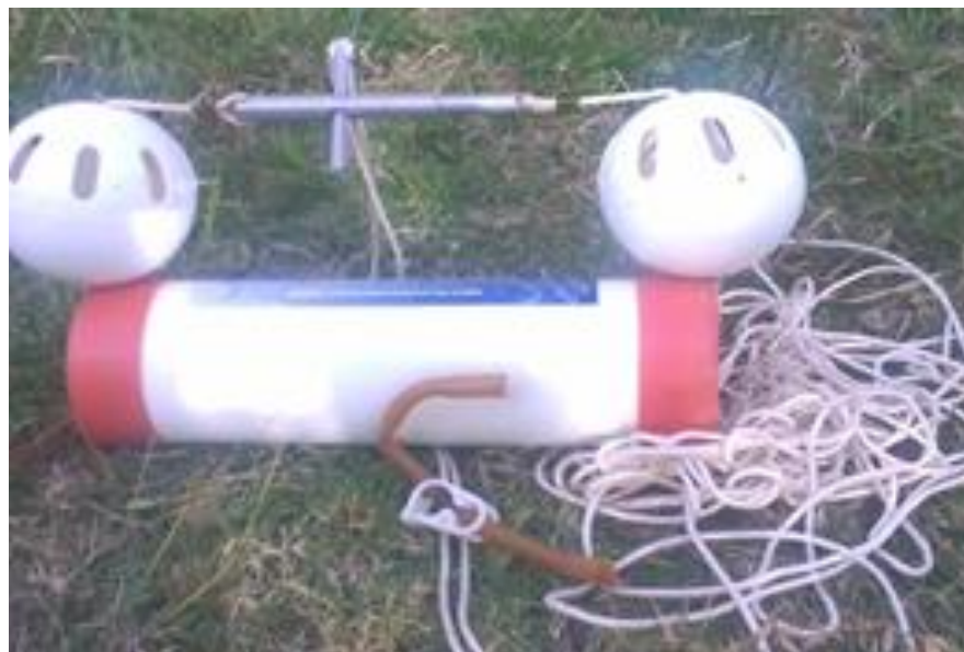
Figure 3. Depth sampler before sampling.
