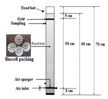
Figure 2. Experimental setup.
