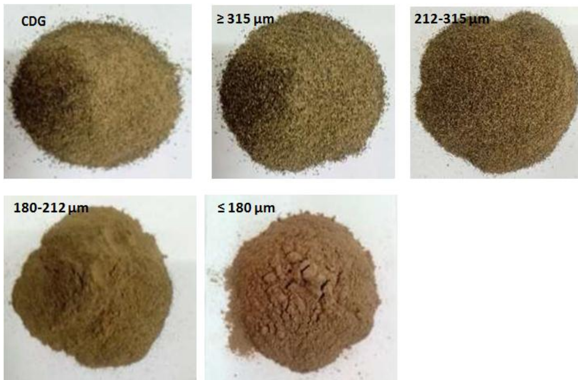
Figure 1. Photos of crude powder (CDG) and CDSP powder fractions from Dichrostachys glomerata fruits. Source: Authors
