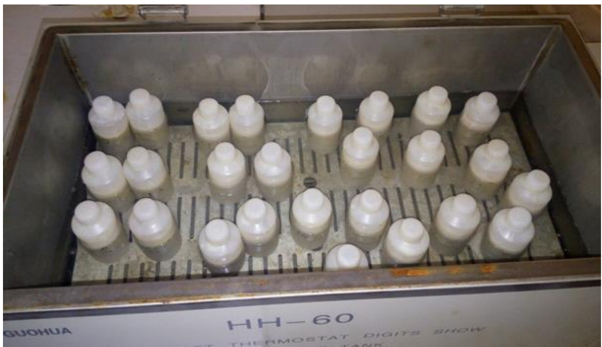
Figure 2. The samples set in Water Bath for pasteurization.
