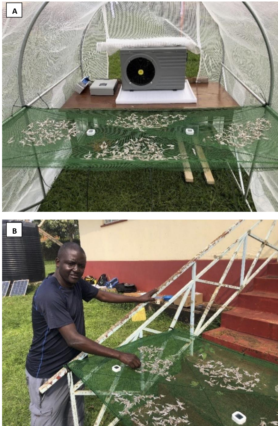
Figure 2. (A) Drying racks inside the enclosure and (B) outside, showing four 100-g samples of fish spread out to dry. The white cubes on the drying racks are SensorBlue temperature/humidity loggers. Source: Authors
