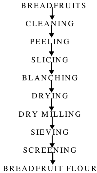
Figure 1. Flow chat for the production of breadfruit flour
