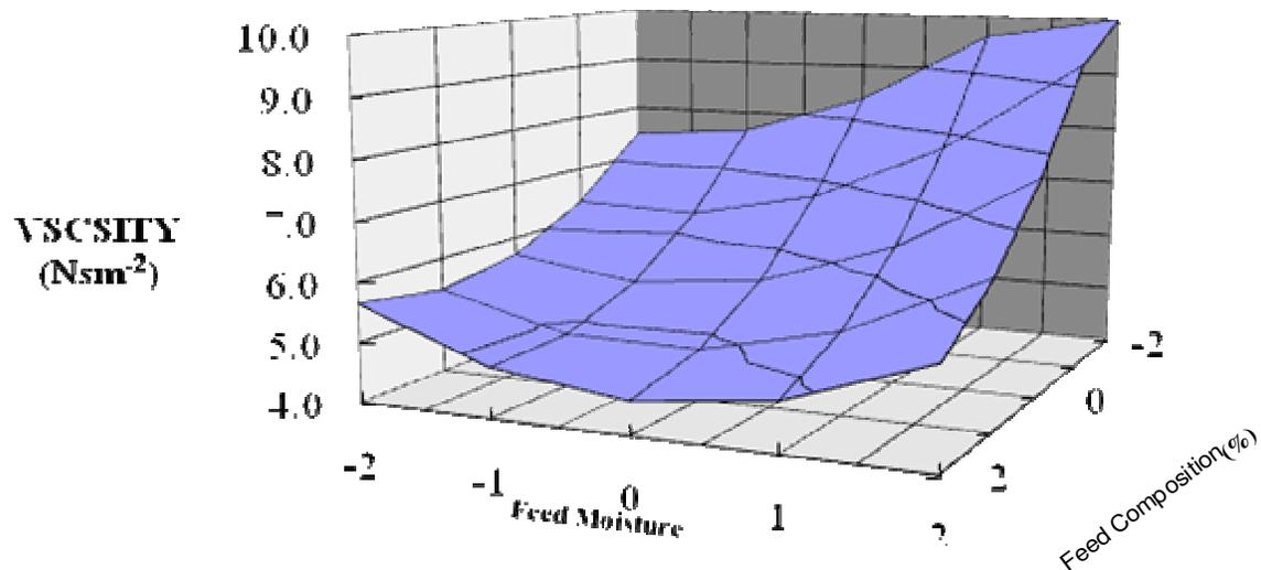
Figure 3. Effect of feed moisture and feed composition on viscosity.
