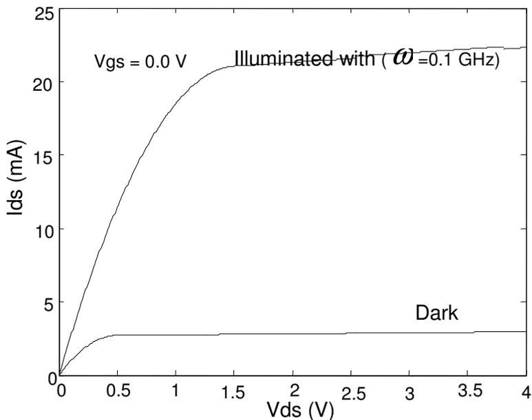
Figure 3. Modulated drain source current verses drain source voltage for  $\lambda= 0.025$ .
