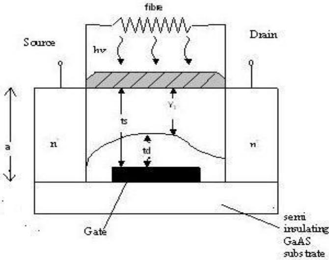
Figure 1. Schematic structure of MESFET.
