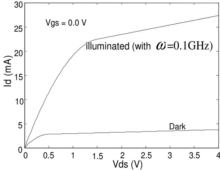
**Figure 2.** Modulated drain-source current versus drain-source voltage under dark and illuminated condition for buried gate structure MESFET at zero gate-source voltage.
