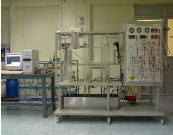
Figure 1. Hardware Set-up of Tank Level Process.
