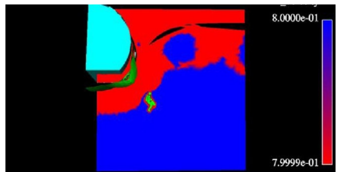
Figure 12. Dichotomous velocity picture: blue \geq 80% free-stream value vs Red < 80% freestream value
