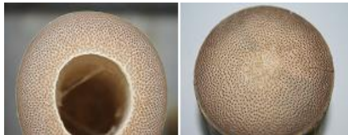
Figure 1. Transversal section of highland bamboo Yushania alpina (left) and lowland bamboo Oxythenanthera abyssinica (Starke, 2014: 3).
