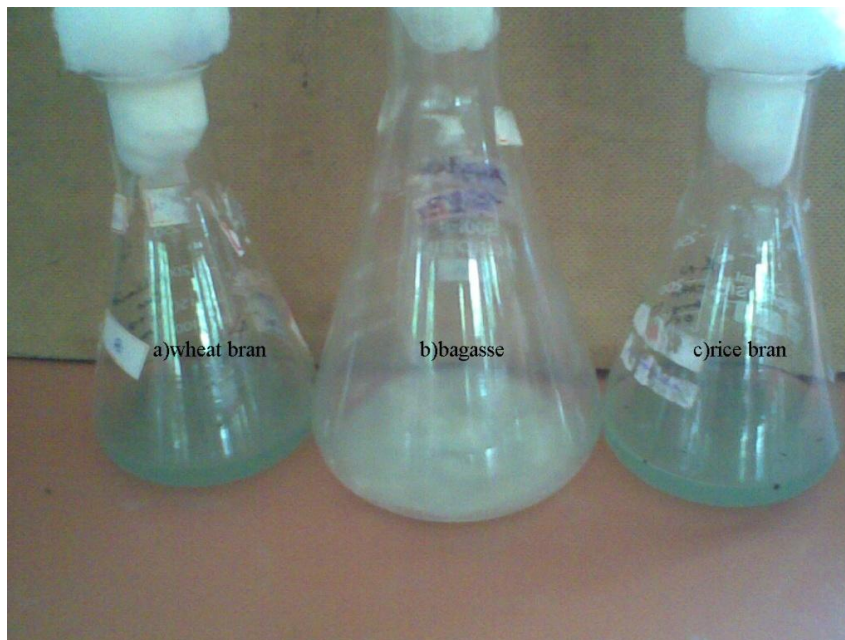
Figure 3. Different substrates (wheat bran, bagasse, rice bran) used in the fermentation medium.
