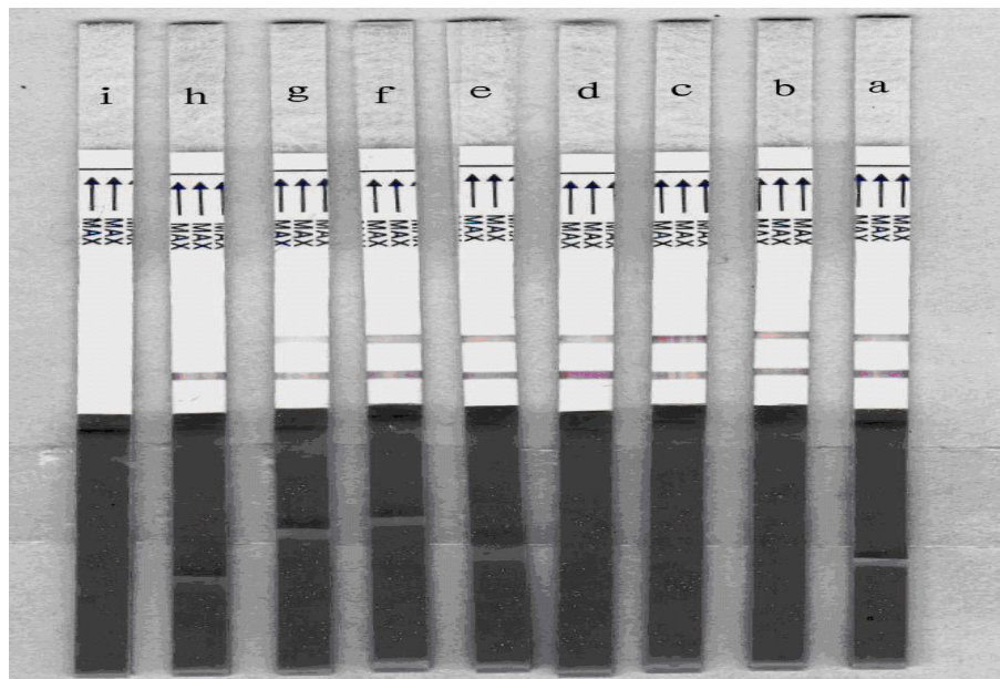
Figure 4. Sensitivity of E. coli O157 immunochromatographic strip with enrichment. E. coli O157:H7 was spiked and then 10-fold diluted from 2.3 \times 10^6 CFU/ml (strip a) to 2.3 CFU/ml (strip g). Strip h was a negative control. The strip could detect 2.3 \times 10^3 CFU/ml before enrichment; it could detect 2.3 CFU/ml (strip g) after enrichment. Strip i was an invalid control.
