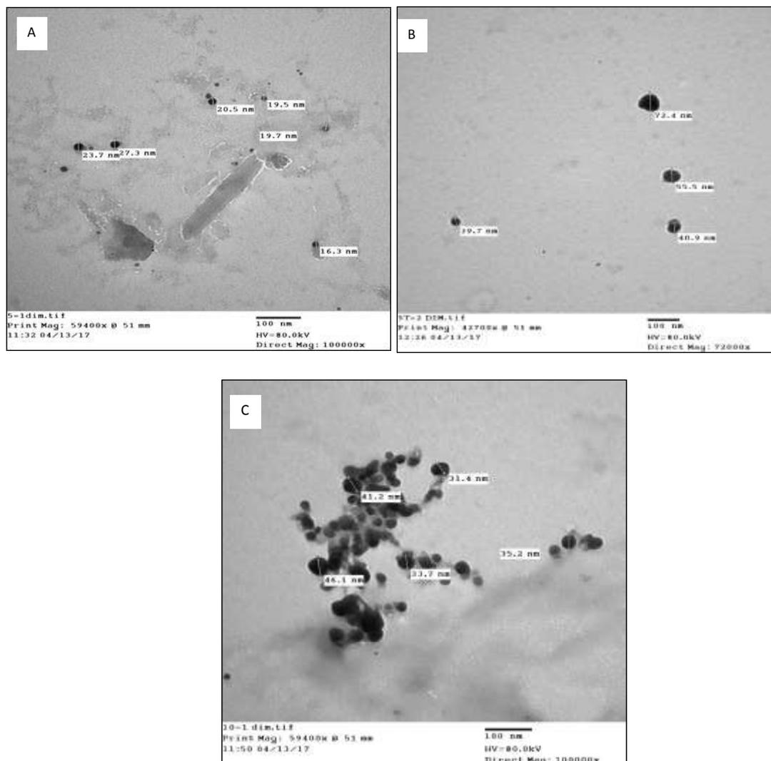
**Figure 2.** TEM micrographs of biogenic AgNPs.
