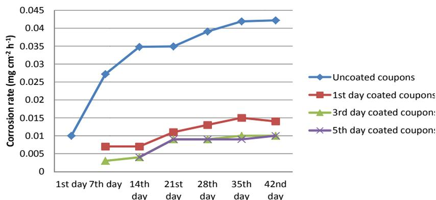
**Figure 3.** Corrosion rate in SRB containing medium at different days with PANI nanofibre coating and without coating.**Table 4.** Inhibition efficiency for PANI nanofibres steel coupons for 1, 3 and 5 days.
