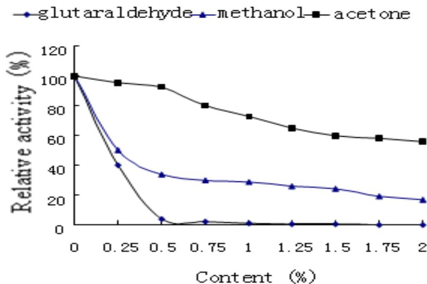
**Figure 4.** Effect of methanol, glutaraldehyde and acetone on xylanase activity. The enzyme was incubated at 55°C for 10 min in 0.067 M phosphate buffer at pH 5.5. The enzyme activity was measured in the presence of methanol, glutaraldehyde and acetone. Values given are the averages of at least three experiments.
