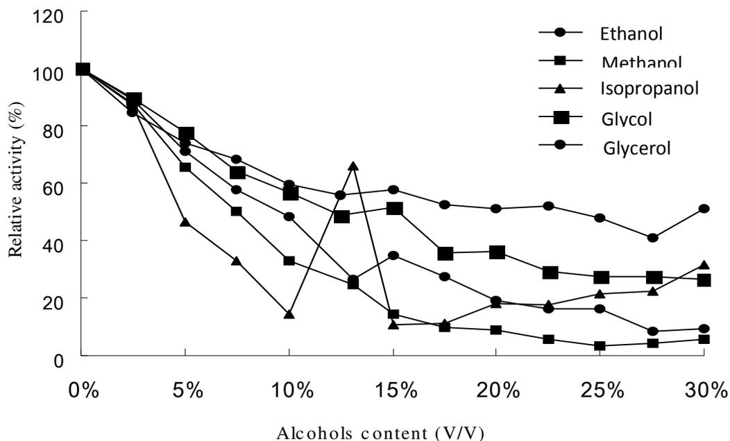
**Figure 3.** Effect of different alcohols on xylanase activity. The enzyme was incubated at 55°C for 10 min in 0.067 M phosphate buffer at pH 5.5. The enzyme activity was measured in the presence of ethanol, methanol, isopropanol, glycol and glycerol. Values given are the averages of at least three experiments.
