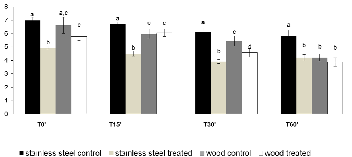
Figure 2. Recovery of Listeria monocytogenes cell loads (log cfu/cm 2 ) inoculated onto stainless steel (washed ■ or not ■ with oregano essential oil) and wood coupons (washed with oregano essential oil ■ or not □ ). The treatment with oregano essential oil was performed for 10 min after that the recovery of the pathogenic strain was performed immediately after treatment (0), after 15, 30, 60 min. For each group considered, different letter represent significant differences (p<0.005).
