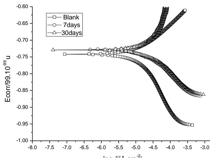
**Figure 4.** Potentiodynamic polarization curves of Q235 carbon steel in cultivated and control system at different growing stages of BF4.
