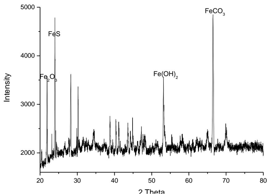
Figure 6. XRD pattern of the corrosion product.
