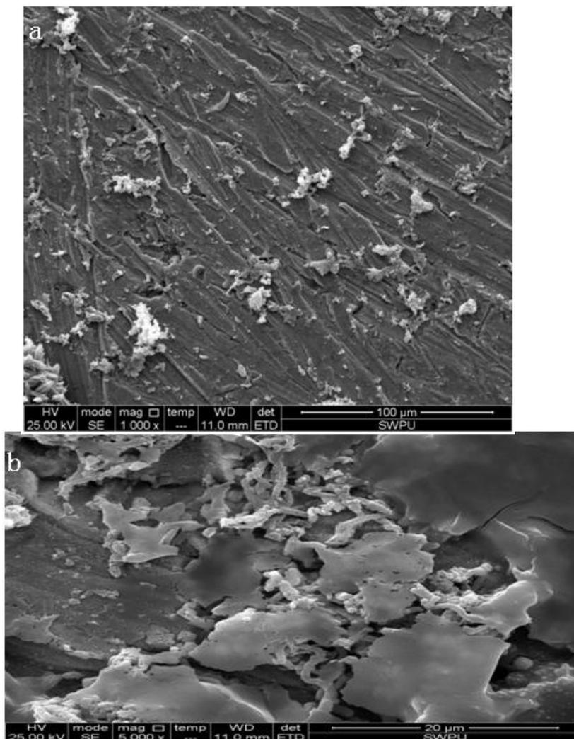
**Figure 5.** Scanning electron micrograph of carbon steel coupon exposed to BF4 (a, b).
