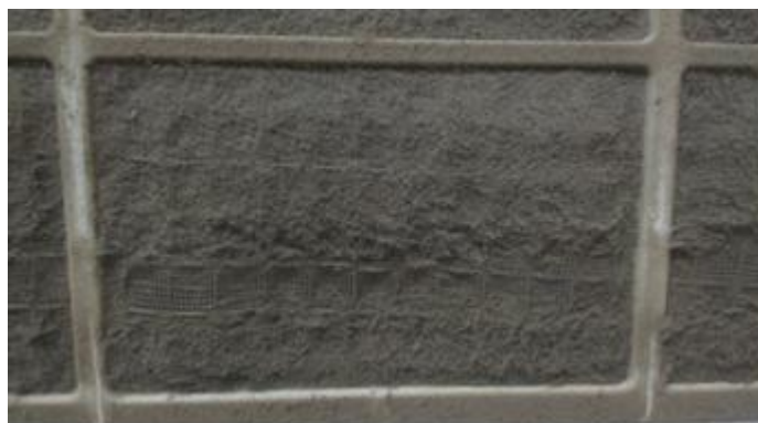
Figure 1. Photograph showing a grossly contaminated filter of the window mounted air-conditioning unit. Source: Author
