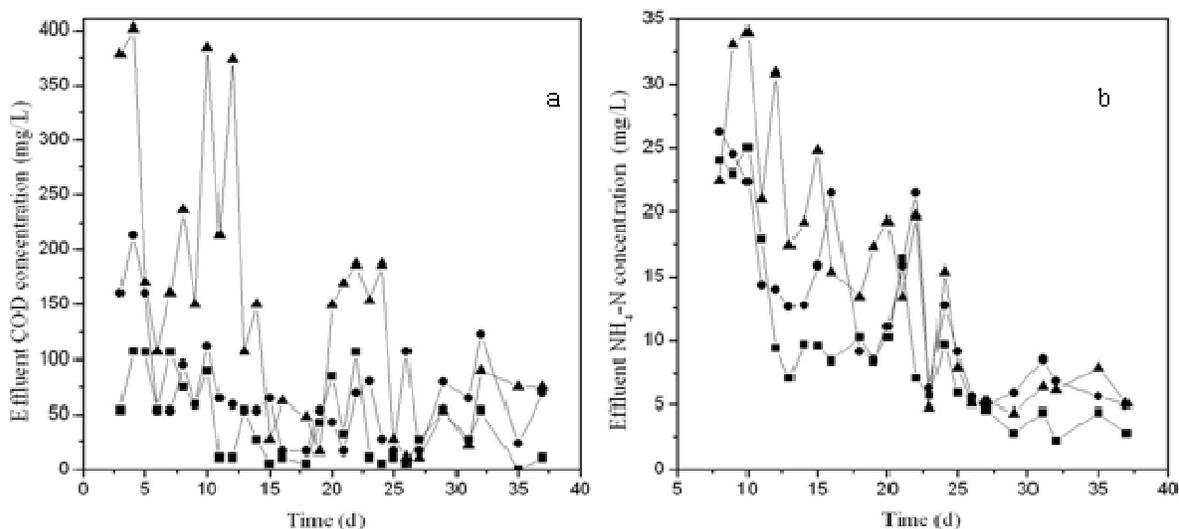
**Figure 1.** Effluent COD (a) and  $\text{NH}_4\text{-N}$  concentrations (b) of M1 (■), M2 (●) and M3 (▲). During the operation the influent COD was about 500, 1000 and 1500 mg/l for M1, M2 and M3, respectively, and the influent  $\text{NH}_4\text{-N}$  was about 25, 50 and 75 mg/l for M1, M2 and M3, respectively. Samples were collected on day 20 and 37.
