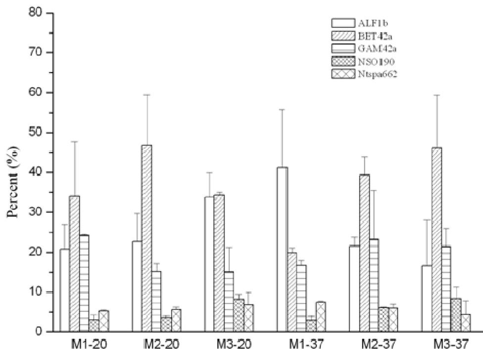
**Figure 4.** Bacterial community analysis of the biofilms in the three reactors as determined by FISH cell counts. The values obtained with the probes ALF1b, BET42a, GAM42a, NSO190 and Ntspa662 were expressed as percentages of the number of cells detected with the probe EUB338. Mn-20, Mn-37: samples collected from Reactor n (1, 2 and 3) after 20 and 37 days of operation, respectively.
