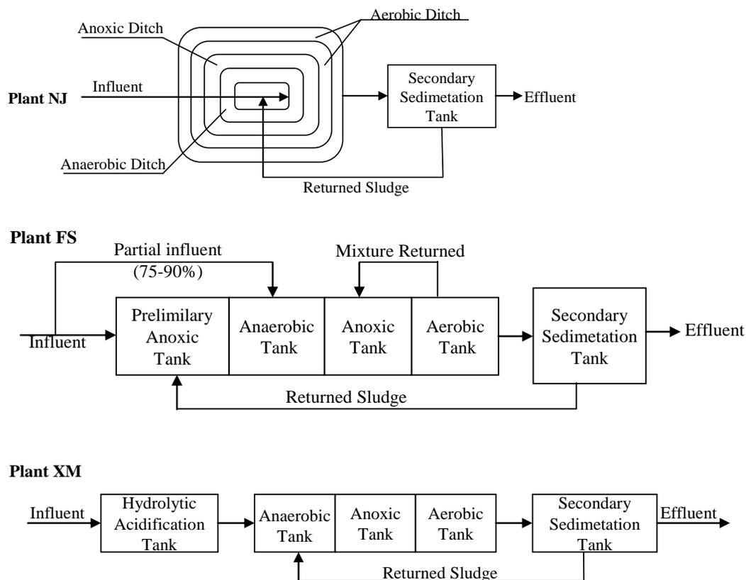
**Figure 1.** The schematic diagram of flow chart of the three MWTPs.
