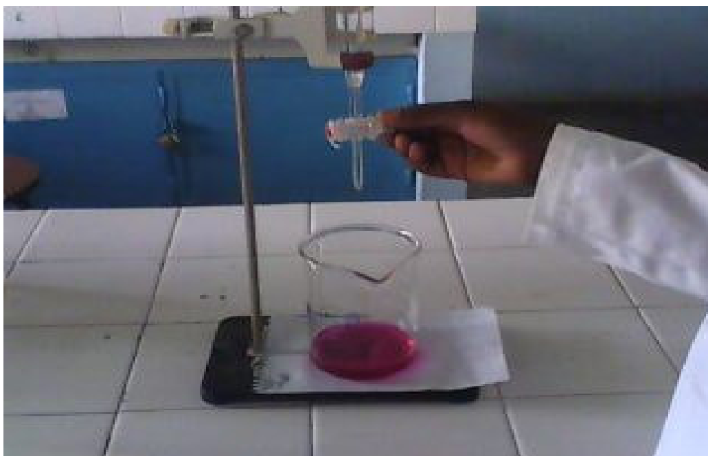
Figure 5. At equivalence point during the titration of citric acid the solution turned into dark pink because of phenolphthalein used as colour indicator.
