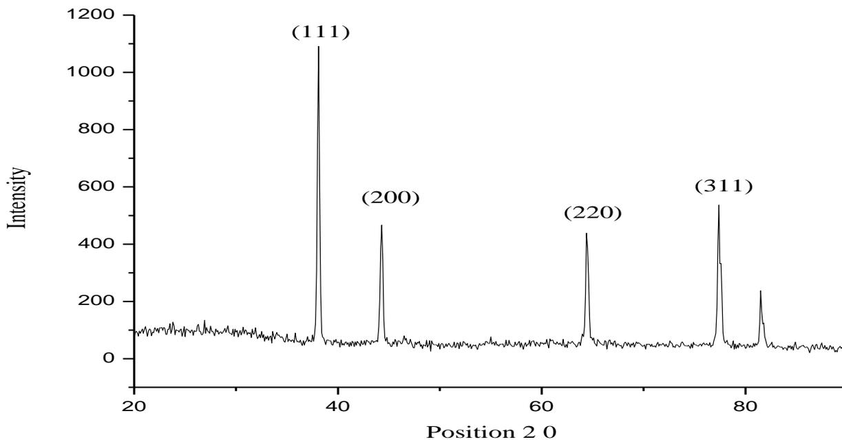
**Figure 6.** X-ray diffraction pattern of the gold nanoparticles.
