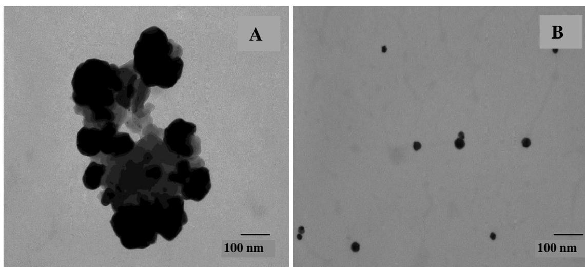
**Figure 4.** Characterization of nanoparticles by transmission electron microscopy: TEM image showing the gold crystals (A) before exposure to  $10^{-4}$  aqueous solution  $\text{HAuCl}_4$ . (B) showing gold nanoparticles (after exposure to  $10^{-4}$  aqueous solution  $\text{HAuCl}_4$ ), synthesized by using *S. hygroscopicus*.
