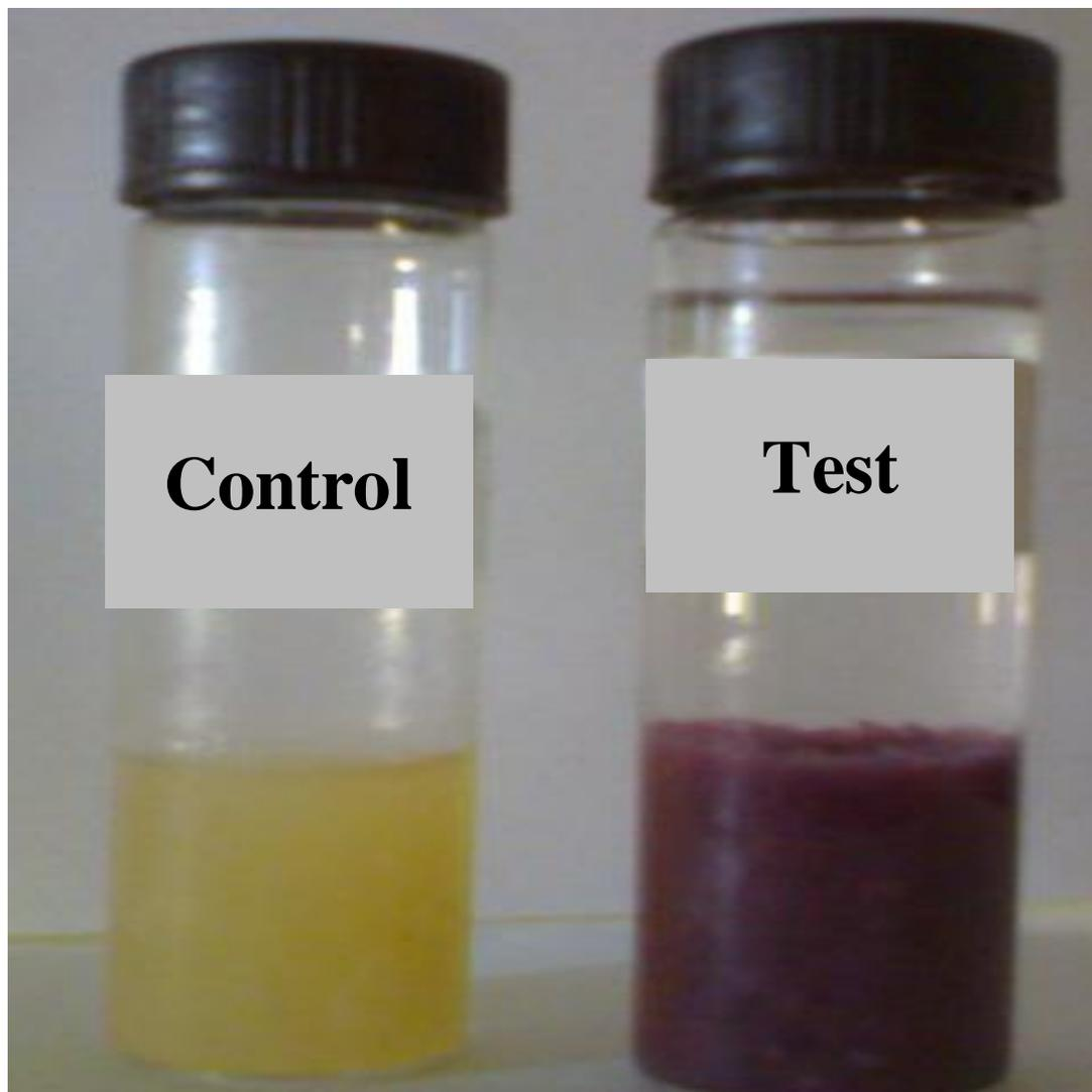
**Figure 1.** *S. hygrosopicus* biomass (control) before exposure to the  $10^{-4}$  mM aqueous HAuCl<sub>4</sub> solution, (test) after exposure to  $10^{-4}$  mM aqueous solution HAuCl<sub>4</sub> for 72 h.
