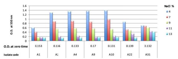
Figure 4. The growth (O.D.550) of the selected isolates at different salinities (NaCl % w/v) after 24 h incubation.
