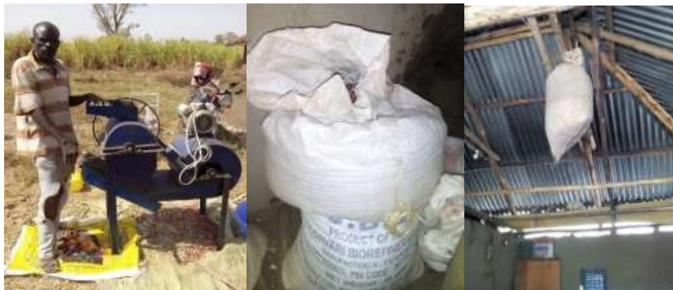
Figure 2. A farmer operating a manually operated groundnut sheller with electric motor and storage containers and place in Homa Bay County.
