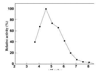
**Figure 9.** pH optimum of *T. harzianum*  $\alpha$ -amylase A3. The reaction mixture contained in 0.5 ml: 1% starch, suitable amount of enzyme and 50 mM sodium acetate buffer (pH 3.6 - 6.0), 50 mM Trsi-HCl buffer (6.5 - 8.5). Each point represents the average of two experiments.
