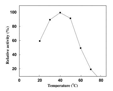
**Figure 7.** Temperature optimum of *T. harzianum*  $\alpha$ -amylase A3. The enzyme activity was measured at various temperatures using the standard assay method as previously described. Each point represents the average of two experiments.
