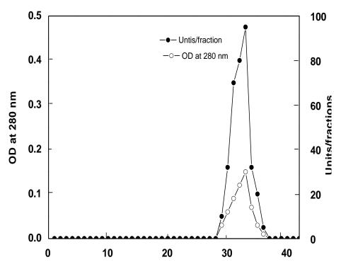
**Figure 4.** Gel filtration of *T. harzianum*  $\alpha$ -amylase A3 DEAE-Sepharose fraction on Sephacryl S-200 column (90 x 1.6 cm i.d.). The column was equilibrated with 50 mM Tris-HCl buffer, pH 7.2 at a flow rate of 30 ml/h and 3 ml fractions.
