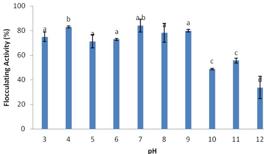
**Figure 9.** Effect of pH on flocculation. Percentage flocculating activity with different letters (a, b, c, d) are significantly ( $p < 0.05$ ) different.
