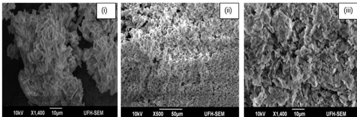
**Figure 4.** SEM images of (i) kaolin clay (ii) biofloculant by *Virgibacillus* sp. Rob (iii) kaolin clay flocculated by the extracted biofloculant.
