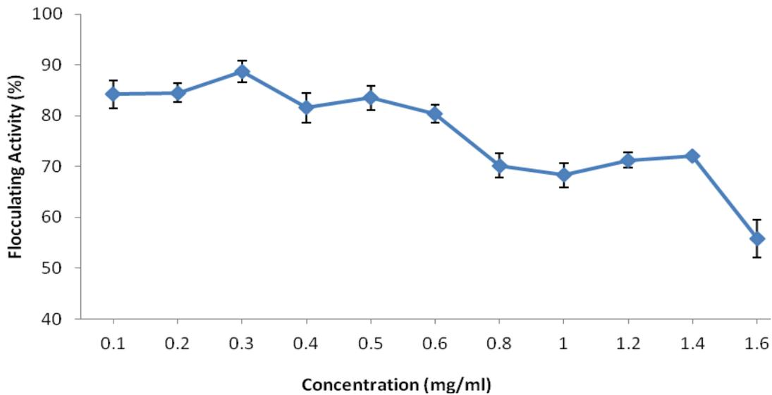
**Figure 8.** Effect of bioflocculant concentration on flocculation. Error bars represent the standard deviation of mean value of
