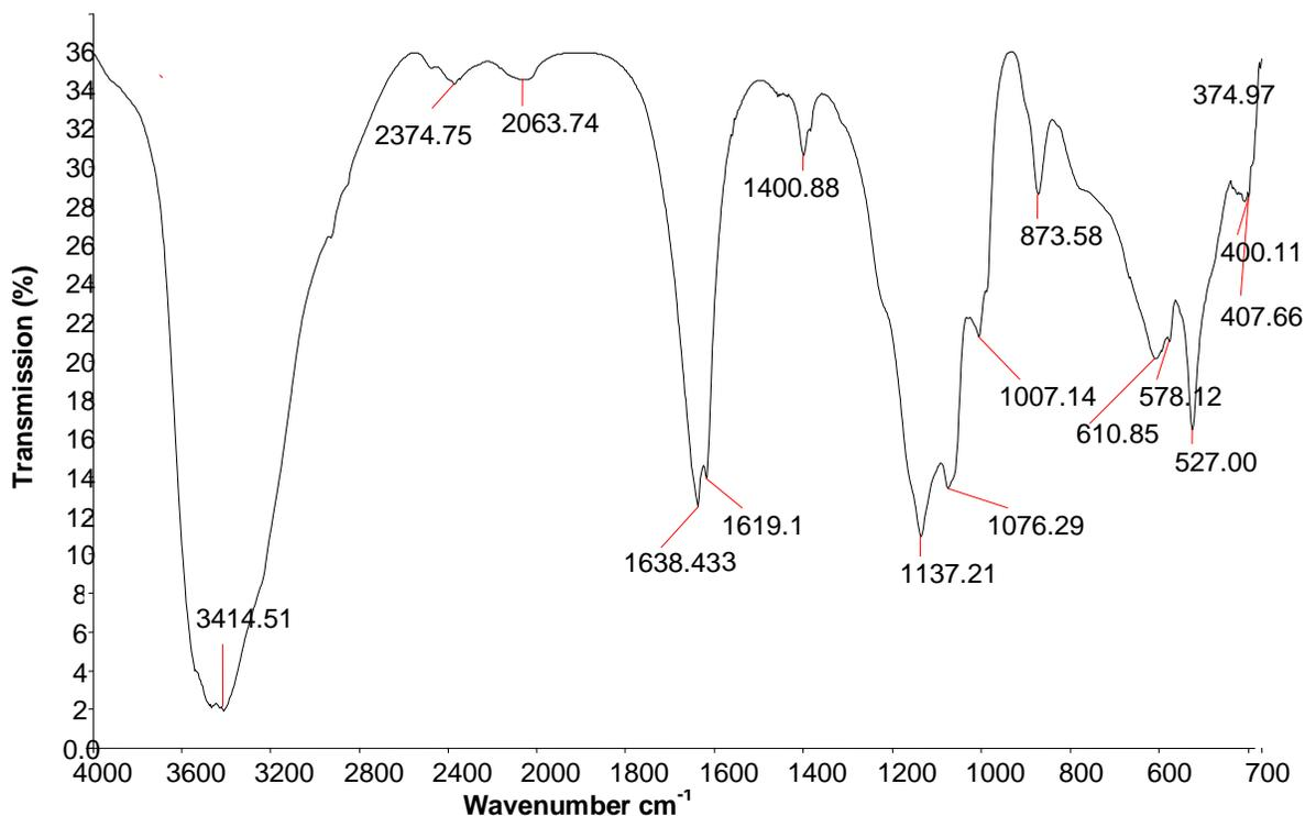
**Figure 5.** Infrared spectra of purified polysaccharide bioflocculant produced by *Virgibacillus* sp. Rob.
