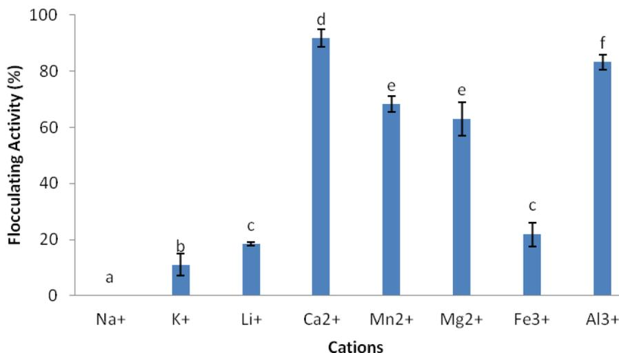
**Figure 10.** Effect of cations on flocculation activity. Percentage flocculating activity with different letters (a, b, c, d, e, f) are significantly ( $p < 0.05$ ) different.
