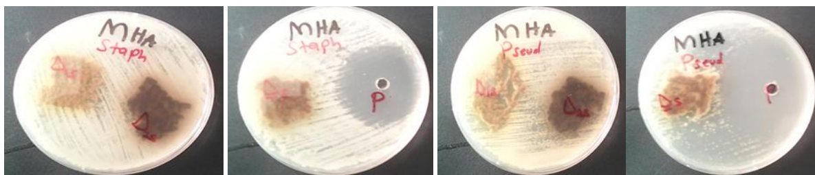
Figure 3. Agar plate pictures of Silk samples dyed with Datura stramonium against Staphylococcus aureus (Staph) and Pseudomonas aeruginosa (Pseud) on Mueller Hinton agar. D 1s -Silk dyed fabric with Alum, D 2s -Silk dyed fabric with Iron sulphate, D s -Silk dyed fabric without a mordant, and P-Control.
