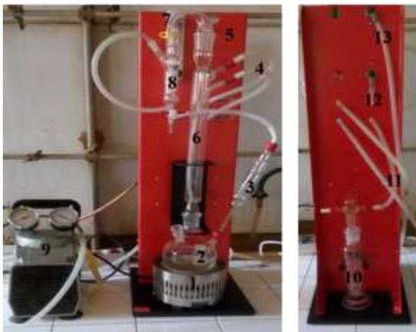
**Figure 1.** KTC, Behr Labor-Technikassure distillation apparatus. 1. Heating device, 2. Round bottom flask, 3. Filling funnel, 4. Water outlet and Water inlet, 5. Support, 6. Condenser, 7. Flow meter, 8. Absorption vessel, 9. Suction pump, 10. Bubbler, 11. Hose to the filling funnel, 12. Hose to the absorption vessel, 13. Hose to the suction pump.
