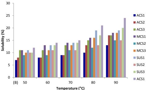
**Figure 3. (a):** Effect of temperature on swelling power of native and modified starches, **(b):** Effect of temperature on solubility of native and modified starches.NAS is Native African Star apple Starch. ACS (1-3) is acetylated starch at 5 (ACS1), 10 (ACS2) and 15(ACS3) g. MCS (1-3) is Carboxymethylated starch at 5 (MCS1), 10 (MCS1) and 15 (MCS1) g.SUS (1-3) is succinylated starch at 5 (SUS1), 10 (SUS2) and 15 (SUS) g.
