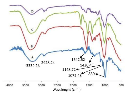
**Figure 5.** The FTIR spectra of native African star apple (*C. albidnum*) kernel starch (A) and a representative acetylated (B), carboxymethylated (C) and succinylated starch (D).
