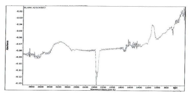
Figure 5. IR spectrum of the corrosion product of mild steel in 0.1 M  $H_2SO_4$  (without inhibitor).
