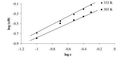
**Figure 4.** Langmuir isotherm for the adsorption of ethanol extract of *Piper guinensis* (EEPG) on the surface of mild steel
