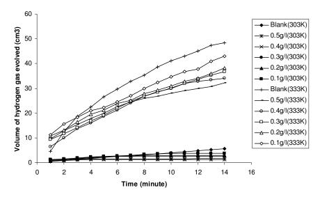
**Figure 1.** Variation of volume of hydrogen gas evolved with time for the corrosion of mild steel in tetraoxosulphate (VI) acid containing various concentrations of ethanol extract of *Piper guineensis* at 303 and 333K.
