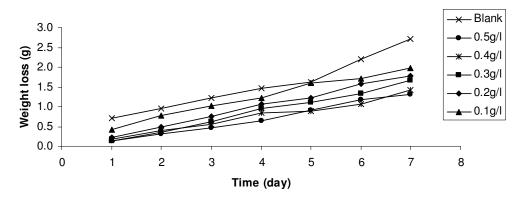
Figure 2. Variation of weight loss with time for the corrosion of mild steel in tetraoxosulphate (VI) acid containing various concentrations of ethanol extract of *Piper guinensis*
