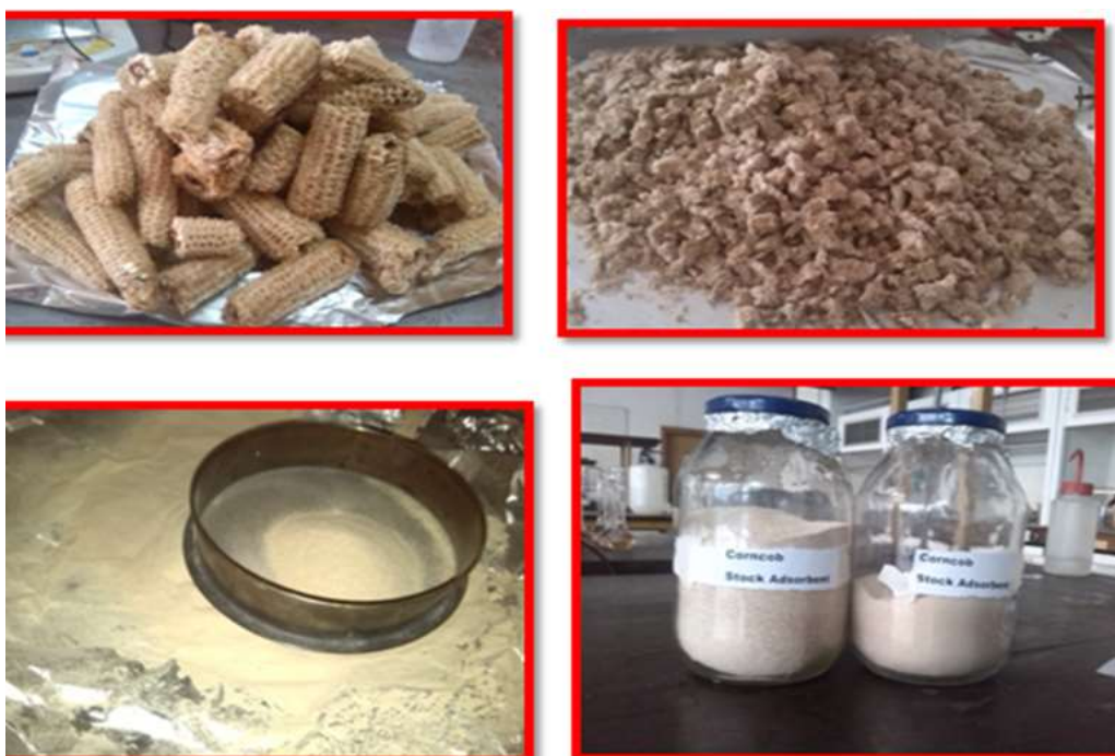
Figure 2. Corncob adsorbent preparation process.
